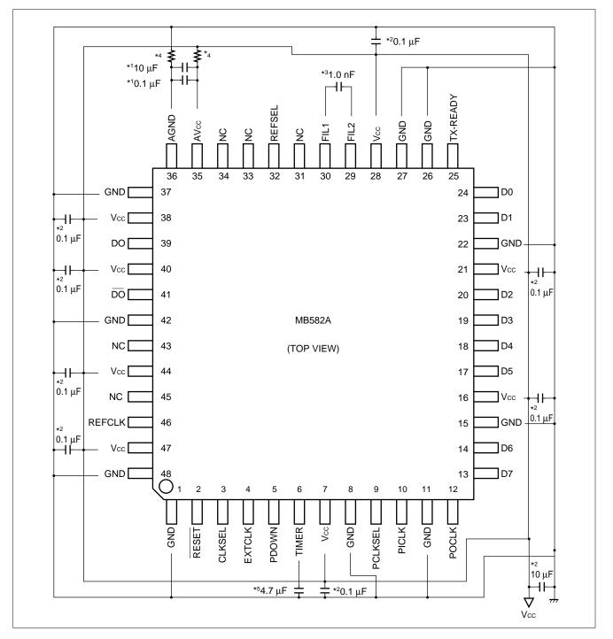
\*1: Bypass capacitor for power supply, connected between analog GND and analog  $V_{CC}$ .
