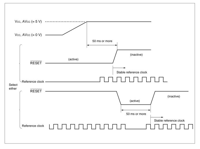
(2) Connect a 4.7  $\mu$ F external capacitor between the TIMER and GND pins. The capacitor is used for automatic power-on reset.
