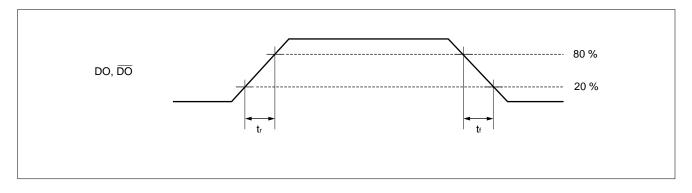
• External serial clock input timing
