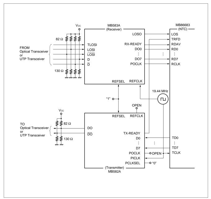
(2) When the MB582A uses PICLK = 19.44 MHz (without REFCLK) and the MB583A uses REFCLK = 19.44 MHz
